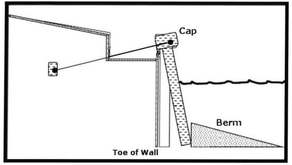
wave action or could occur if the panels are not buried sufficiently in the bottom or the berm is improperly placed. Observable symptoms include cap rotation, movement, or cracking; an opening gap between the bulkhead and an existing dock or any support pilings built tightly against the bulkhead. Potential remedies include:
