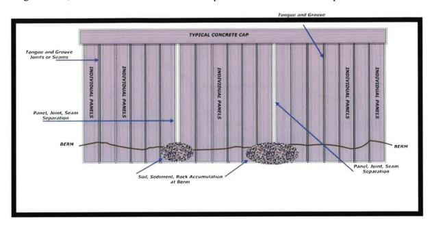
Observable symptoms include sinkholes, visible separation in seams (found by a diver), or sediment underwater at the base of an affected joint. Remedies may include:
