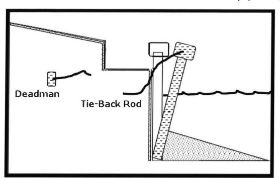
include a deteriorating cap with cracks or spalling, wavy or sagging panels, and backfill settlement. The results include rotation of the cap away from the land and toward the water, crumbling of the cap and loss of its ability to keep panels aligned or vertical. Remedies may include:
