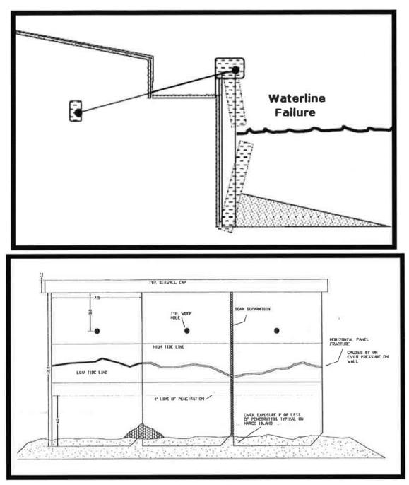
and the panels will eventually break along those lines. In this situation the affected sheet panels must be replaced and the tiebacks either replaced or supplemented with helical tiebacks.
